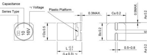
\*1. Voltage mark for 6.3V is [6V]      6.3V 的產品標識為 [6V]
